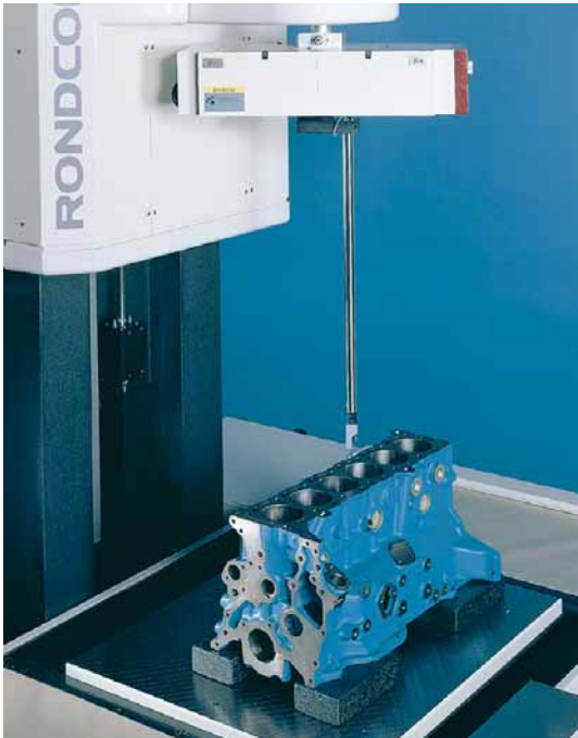
Examples of typical applications for Rondcom 72/76: measurement of cylinder heads, engine blocks and crankshafts
