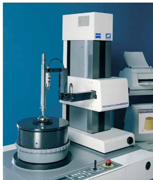
Rondcom 55 with fully-automatic rotary table
